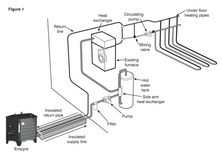
**Note:** The installation of the Empyre as an add-on unit must be installed without changing the function of the controls or rewiring the original boiler. A wiring interconnection is permitted. The electrical system of both boilers must be powered from a single branch circuit without exception.
