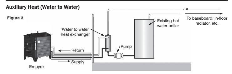
A regular furnace system is left intact and automatically cuts in when the Empyre Outdoor Wood Furnace runs out of wood, Figure 3.
